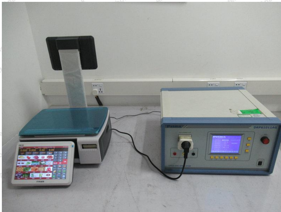
Photo of Voltage Dips and Interruptions Test
