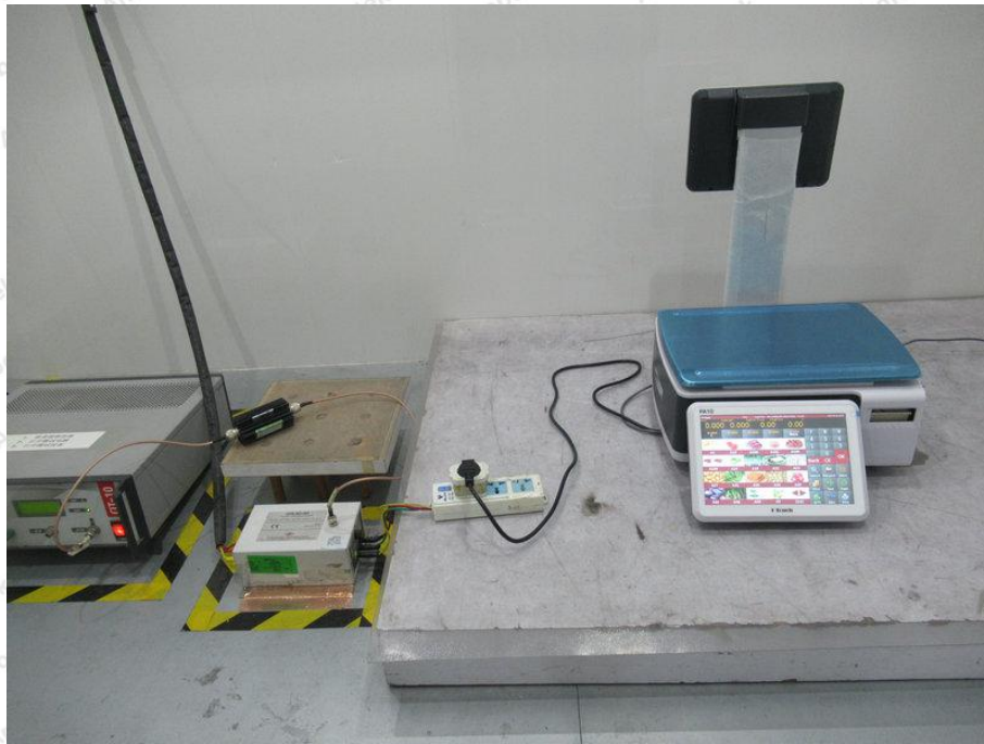
Photo of Injected currents susceptibility Test
