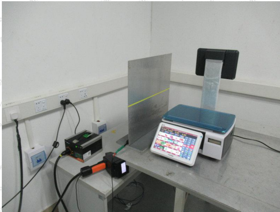
Photo of Electrostatic Discharge Immunity Test
