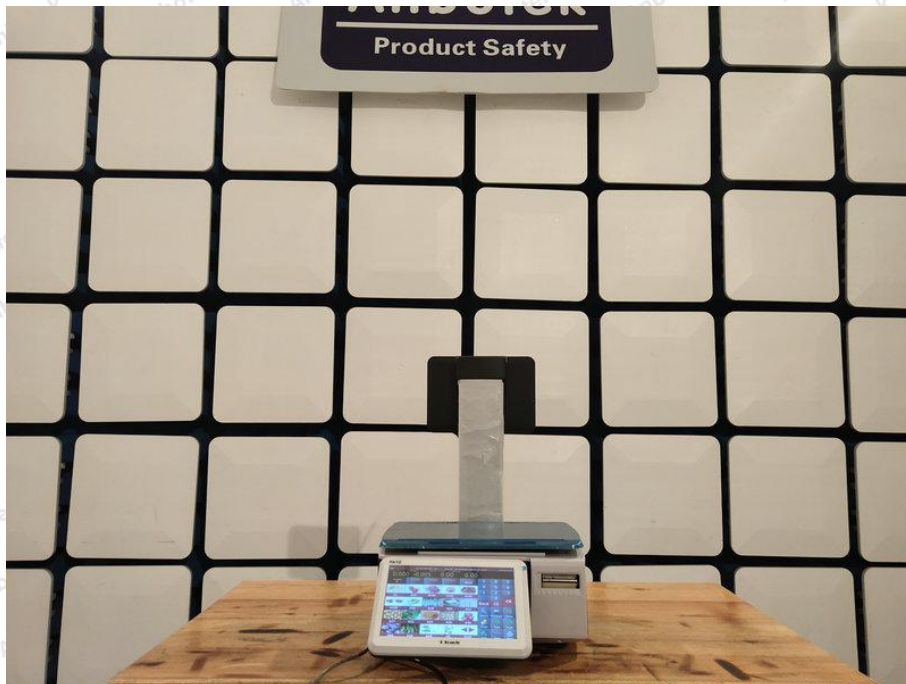
Photo of RF Field Strength susceptibility Test
