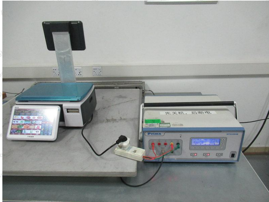
Photo of Electrical Fast Transient/Burst Immunity Test
