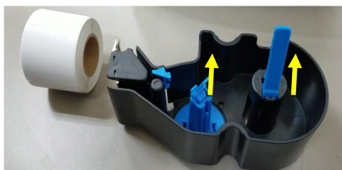
④ Release stopper levers then Remove back paper roll and label core
